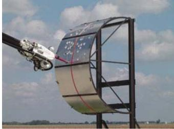
Penetrating between the holes can extend panel usability; however, doing so enough times can create very large holes that can lessen the uniform tightness of that panel thus reducing the quality of the penetrations. Also, doing so can cause bits of aluminum to fall to the ground. The fallen pieces should be picked up to prevent them from possibly becoming foreign object damage (FOD) candidates. Those pieces are sharp, so they should be handled using gloves.
